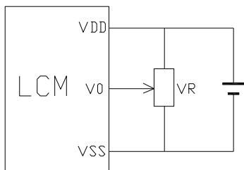
V<sub>DD</sub>-V<sub>0</sub>: LCD Driving voltage
