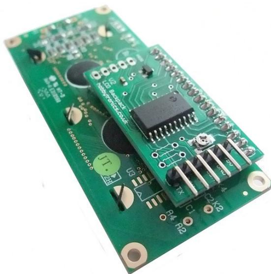
The six pin (straight or right-angle) header pins should be soldered on first
